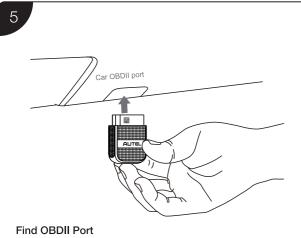
Plug the connector of the Bluetooth dongle into the vehicle's OBDII port.
